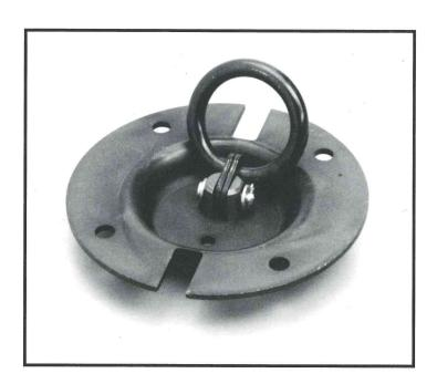
Pan Fitting with articulated ring — This heavy duty fitting was designed and developed for military applications. This pan fitting meets the standards established in MIL Std-209 for Class 4, 5000 lb. tiedowns. It's made from 4130 heat treated alloy steel and zinc plate Olive drab. The fitting has a breaking strength of 7,500 lbs. and a working load rating of 2,500 lbs.
