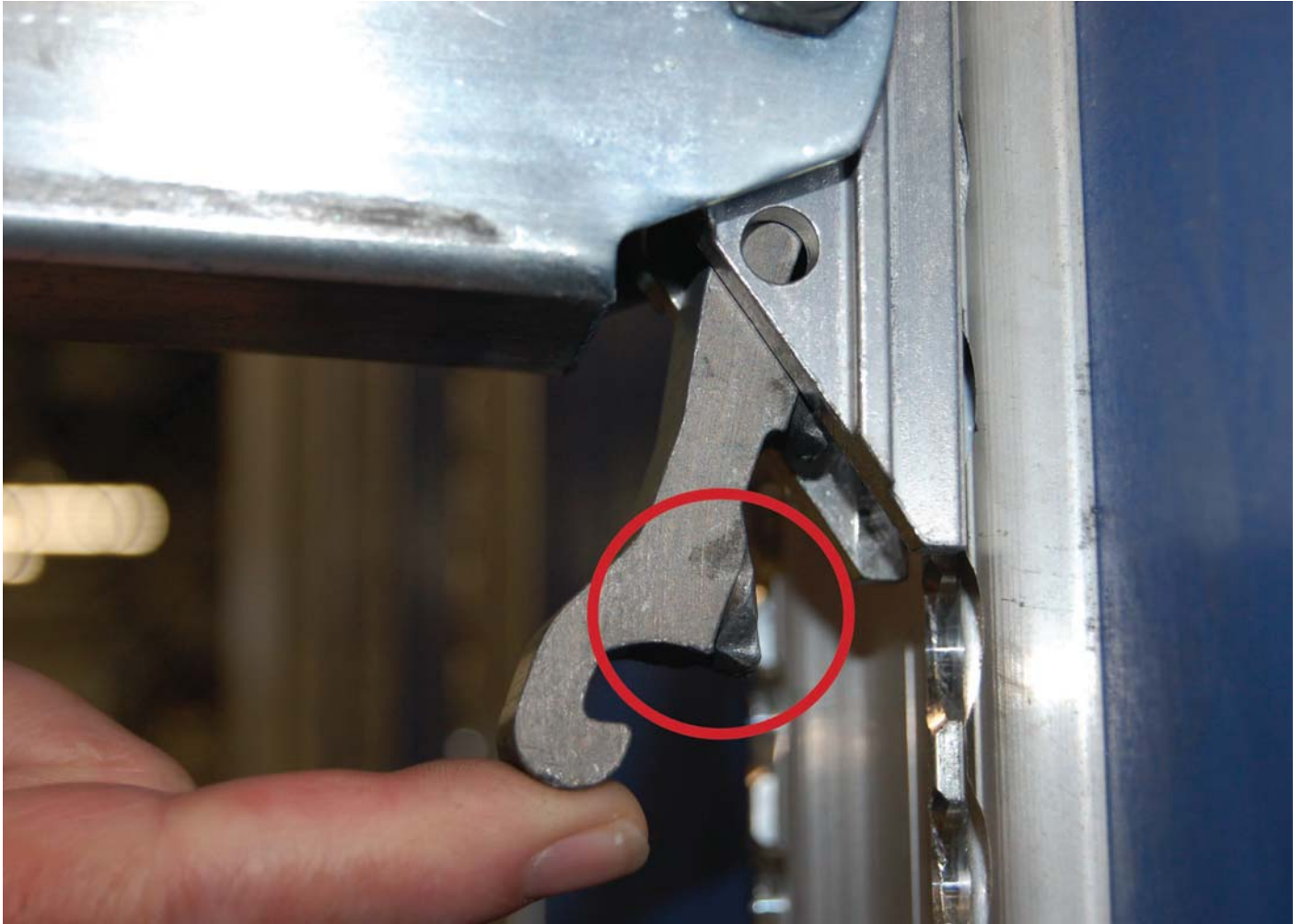
Excessive Wear on LAD II Beam Foot Lock Key
