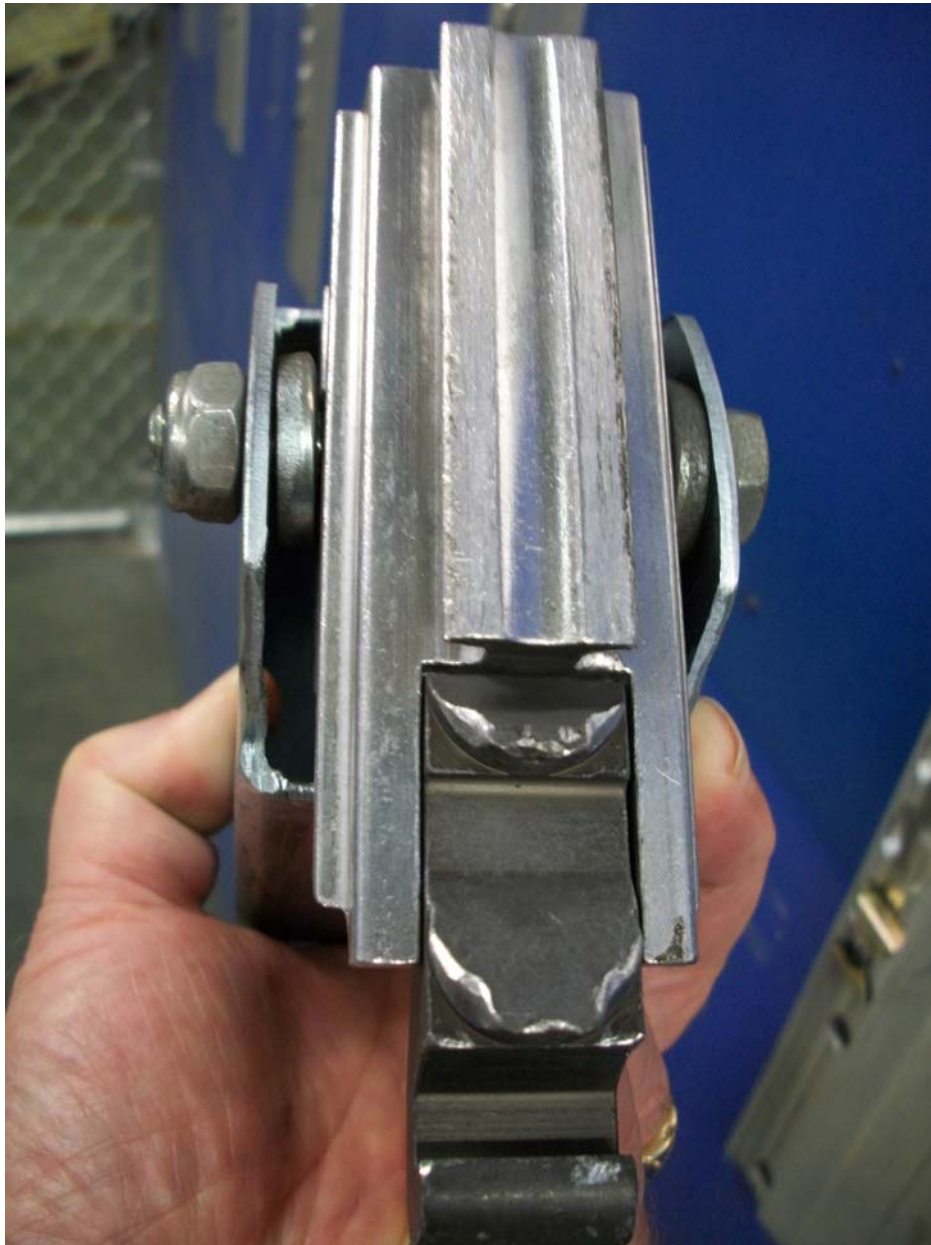
Excessive Wear on LAD II Beam Foot Lock Key
