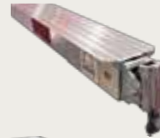
50587-10 Wide Top Low Profile Beam Assembly WLL: 3,000 lbs./1360 kg. Max Cargo: 750 lbs. / 340 kg. Length: 98"-113.4"/ 249 to 288 cm.
