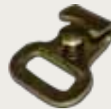
40044-10 1-inch Flat Hook with Keeper WLL: 1,166 lbs./530 kg. Weight: .68 lb./31 kg.
