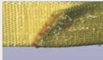
Broken or worn stitching in load bearing sew patterns
