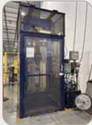
TENSILE TEST MACHINE – Checks Ancra webbing and hardware for load capacity using up to 50,000 lbs of force
