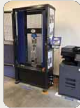
ADMET MEASUREMENT SYSTEM – It is used for evaluating compression and positive force load testing with an Ancra designation of ETF-614 / QC-18
