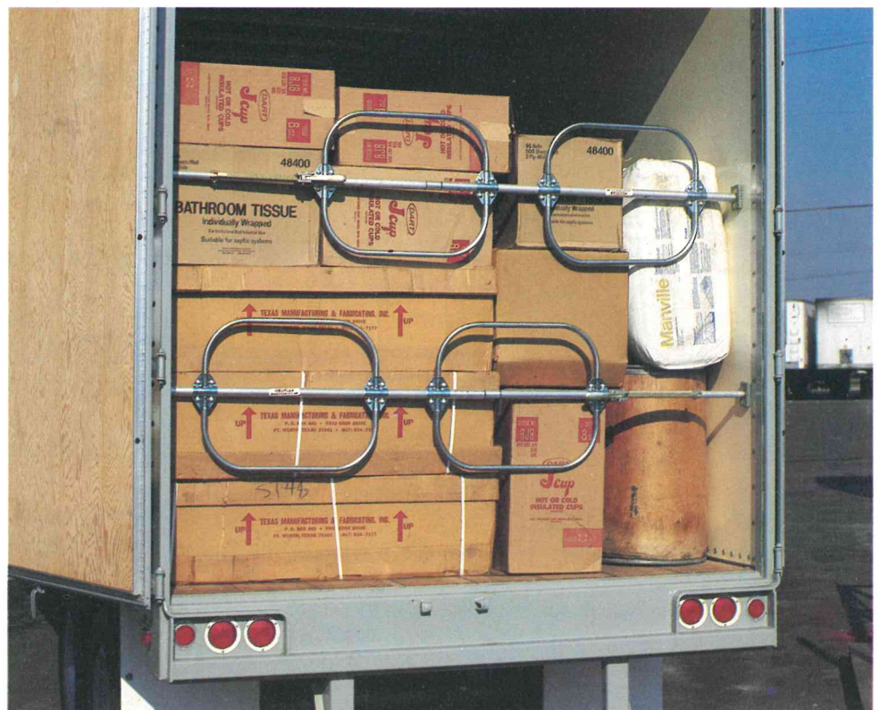
Cargo Hoops, in sets of two, are mounted to Cargo-Sta for effective retention of small packages.
