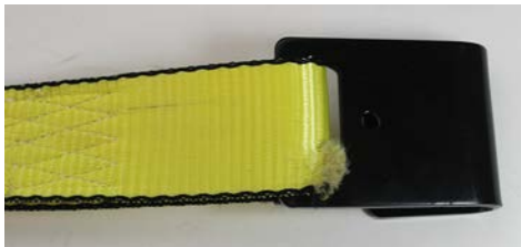
Figure 8 Tear in Webbing at the Fitting.
