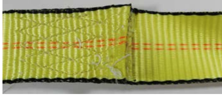
Figure 2 Broken or Worn Stitching in Load Bearing Sew Patterns.
