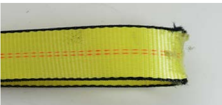
Figure 7 Damaged Loop, Eye Hook Too Small or too Rough.
